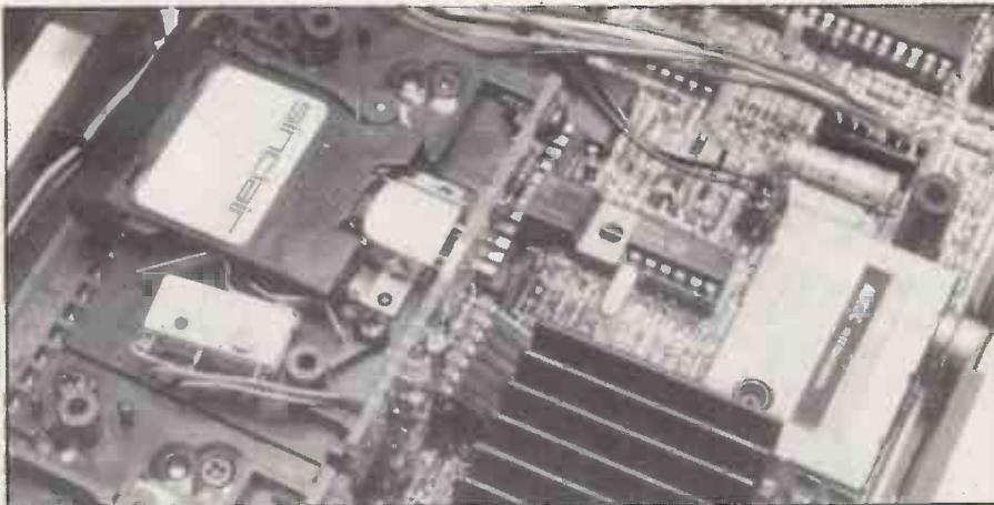
When the Microdrive cartridge slots in the tape is pressed against the read/write head.
